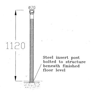
steel grade = S 275 post size = 48.3 mm diameter x 5 mm thick
