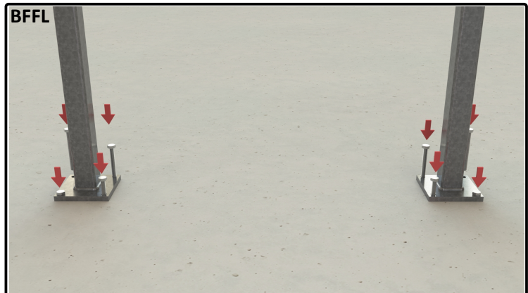
02b) Using suitable fixings install the primary posts. The primary posts must be perfectly aligned and vertical for the glass gate to function optimally.
