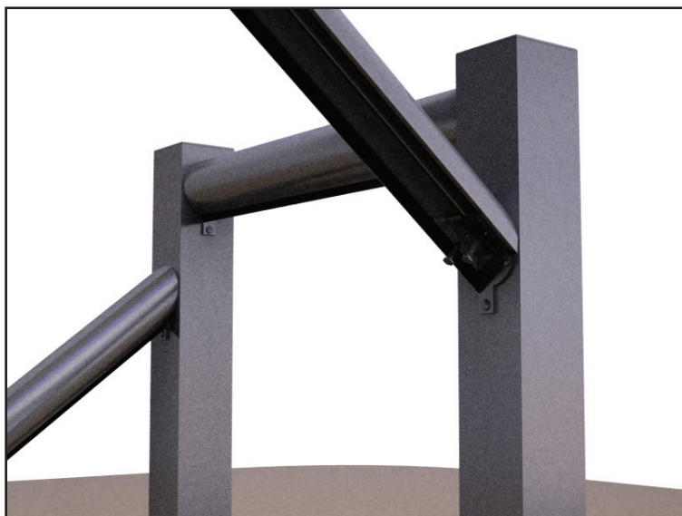
21 Drill 4mm holes through brackets into the handrail
