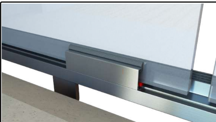
11) Install the bottomrail and handrail glazing bead bits and wedge gasket to hold the glass panel(s) temporarily.
