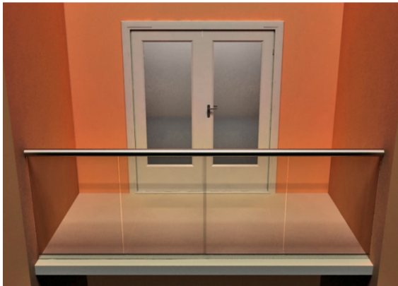
Balcony 1 Balustrade fixed between two walls
