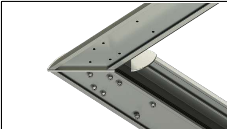
03) Fix the corner bracket to the Aerofoil handrail with seven 4.8x19mm socket cap self tapping screws.
