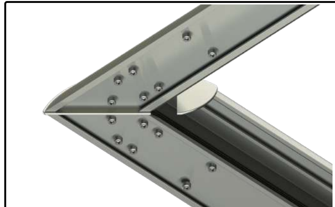
06) Fix the corner bracket to the Infinity handrail with seven 4.8x19mm socket cap self tapping screws.
