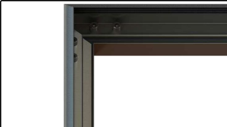
31) Fix the bottomrail connector to the bottomrail with two 4.8x13mm socket cap self tapping screws.
