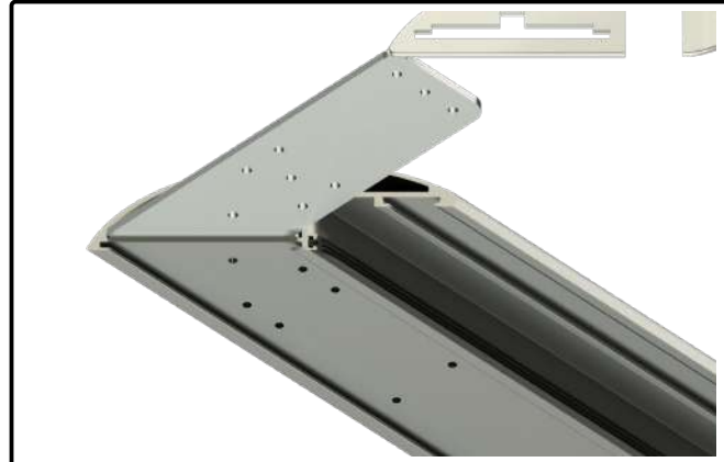
02) Slide the corner bracket into the Aerofoil handrail.
