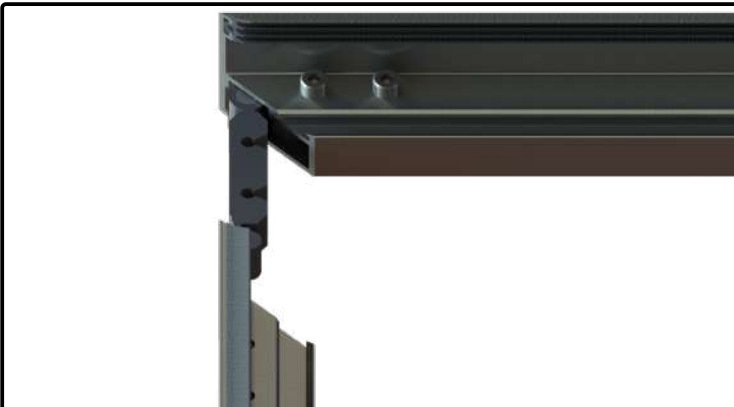
29) Fix the bottomrail connector to the bottomrail with two 4.8x13mm socket cap self tapping screws.
