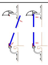
10) Seat a glass panel onto the packers and pivot the panel up to make contact with the fixed (E) gaskets.
