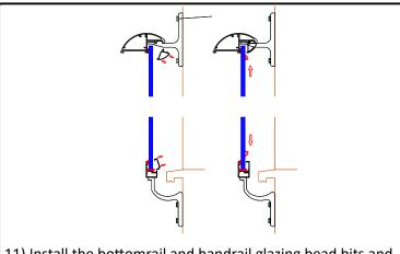
11) Install the bottomrail and handrail glazing bead bits and wedge gasket to hold the glass panel(s) temporarily.
