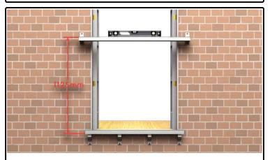
05) Measure the 1125mm from the underside of the bottomrail. Position the handrail centrally and level over the opening.
