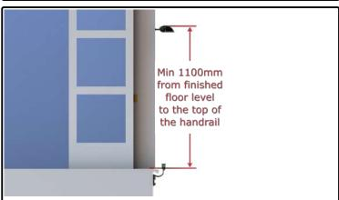
06) Ensure the handrail is at a minimum of 1100mm from the finished floor level.
