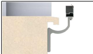
03) Position the bottomrail to give access to install the glazing bead so that a standard system height of 1125mm (underside of the bottomrail to the top of the handrail) achieves a minimum of 1100mm from the top of the handrail to the finished floor level.
