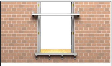
07) Once positioned correctly mark the fixing locations and with suitable fixings fix the handrail to the structure.
