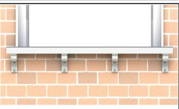
04) Once positioned correctly mark the fixing locations and with suitable fixings fix the bottomrail to the structure.
