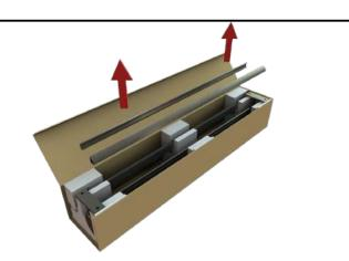
01) Unpack your Juliet, remove the handrail and bottomrail glazing beads and place to one side.
