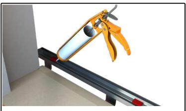
08) Stick two 5mm glass packers per glass panel into the bottomrail with a blob of silicone.
