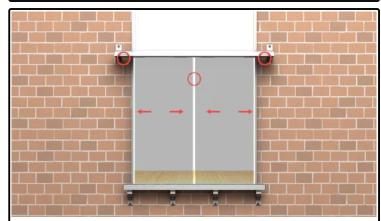
14) Adjust the glass panels and gaps as required.
