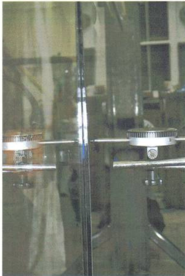
Plate No.7 A close up view of displacement monitoring equipment (dial test indicator) required to record the maximum displacement of each balustrades component feature under loading.
