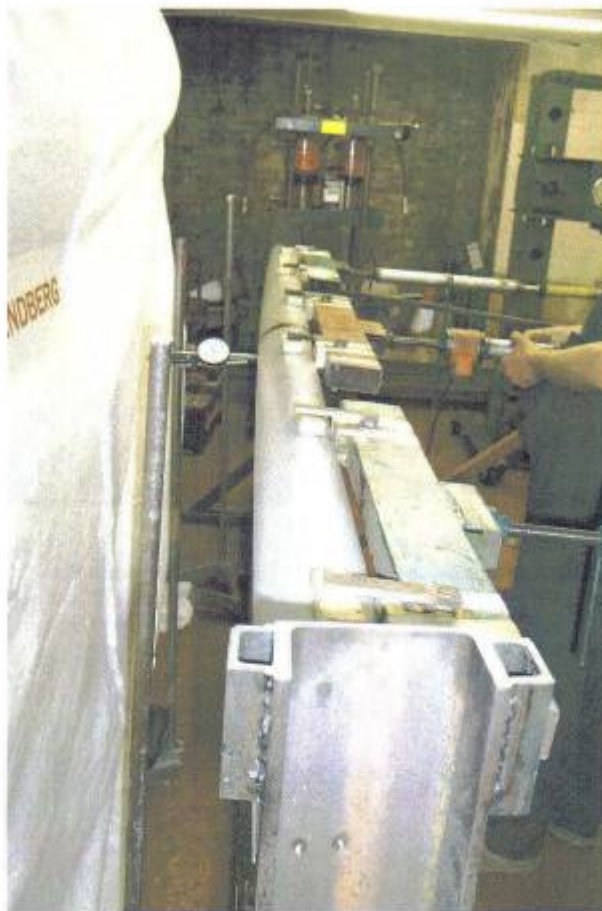
Plate No.2 Showing a view along the hand rail feature of balustrade system No.1 during application of the test force showing the handrails progressive resultant displacement under loading.
