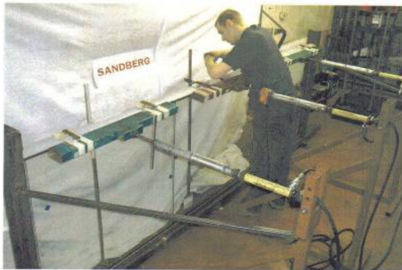
Plate No.1 A view of the balcony balustrade system (No.1) during preparation for testing under the horizontal uniformly distributed line loading at 0.74 \text{ kN/m} run.
