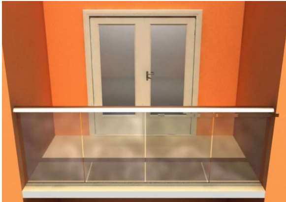
Balcony 2 Balustrade fixed between two walls
