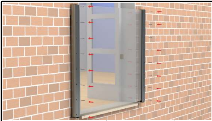
17) Clamp the glass in place by fixing the pusher profiles to the base profiles with the provided sixteen 4.8 x 38mm self tapping screws, eight per pusher profile.
