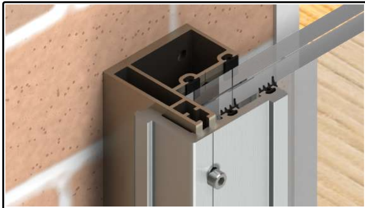
18) The glass is now fully supported.
