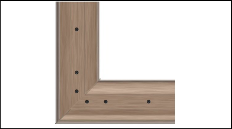
6) Tighten the screws. In this fashion assemble all the handrail parts and sections together.
