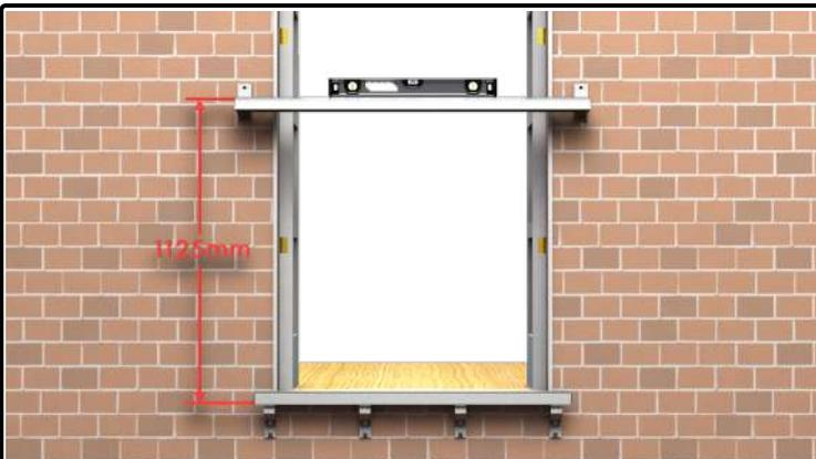
05) Measure the 1125mm from the underside of the bottomrail. Position the handrail centrally and level over the opening.
