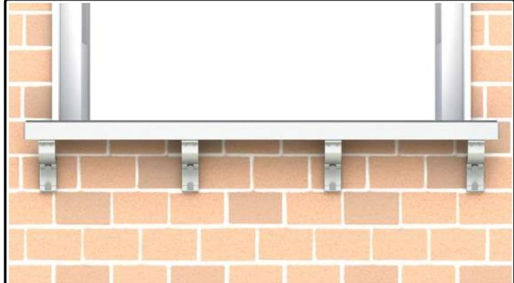
04) Once positioned correctly mark the fixing locations and with suitable fixings fix the bottomrail to the structure.
