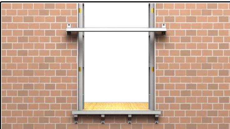
07) Once positioned correctly mark the fixing locations and with suitable fixings fix the handrail to the structure.
