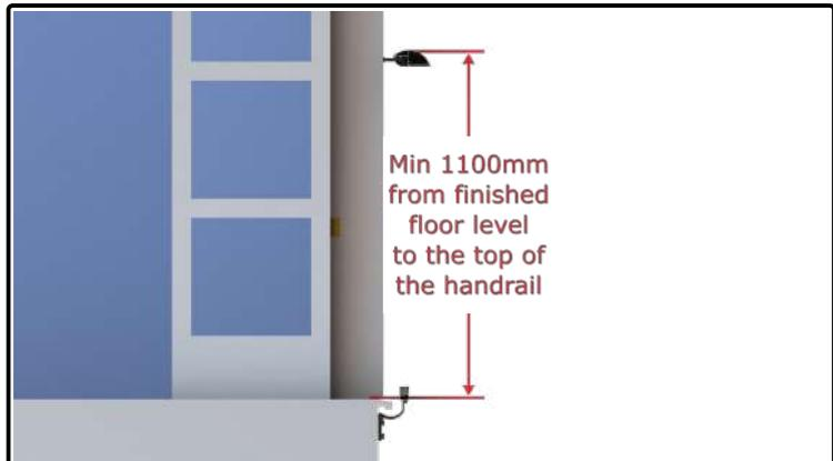
06) Ensure the handrail is at a minimum of 1100mm from the finished floor level.
