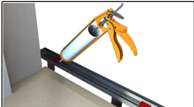
08) Stick two 5mm glass packers per glass panel into the bottomrail with a blob of silicone.
