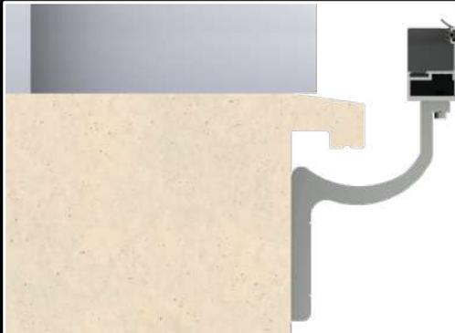
03) Position the bottomrail to give access to install the glazing bead so that a standard system height of 1125mm (underside of the bottomrail to the top of the handrail) achieves a minimum of 1100mm from the top of the handrail to the finished floor level.
